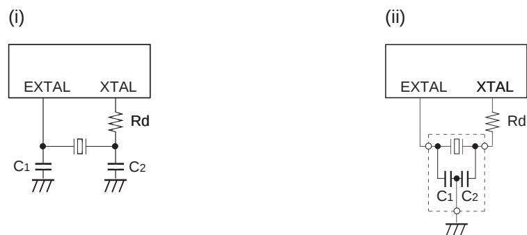
Fig. 13. Recommended Oscillation circuit
